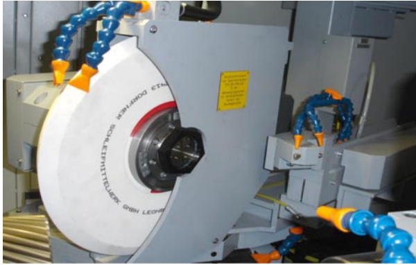
An example of an external and surface grinding unit at an angle of 45° in relation to the work-piece axis with external and surface grinding wheel profiled on both sides
