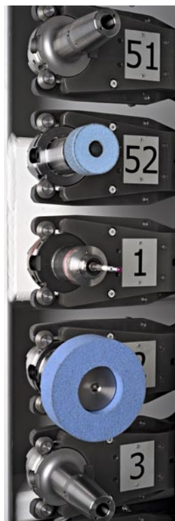
An example of a 52-fold tool changer, with the changing process being intended for the complete processing of complex components in one clamping
